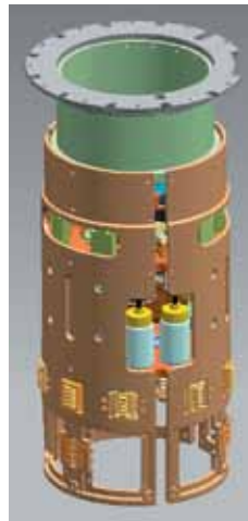
Fig.13 Diverter switch
